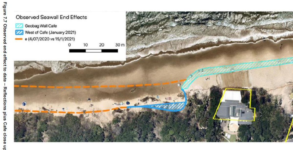
Figure 12 Observed end effects from combined geobag structure (WRL report)
